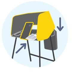
Voter casts ballot into Integrated Ballot Box attached to the Ballot Marking Device
